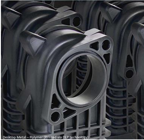
Desktop Metal – Polymer (Printed via DLP technology)
