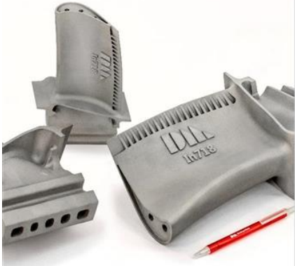
Desktop Metal – Metal (Printed via Binder Jet technology)
